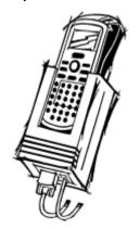
Battery charging and/or communications cradle designed for in-transit applications. Mounted inside a vehicle, this cradle provides connectivity to any RS-232 serial device including printers, radio modems, GPS, on-board computers and vehicle monitoring systems.
